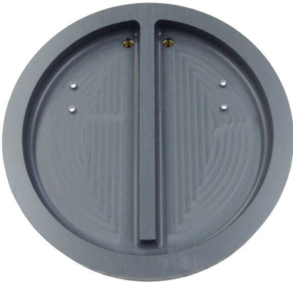
Fig. 5 Hard Surface Emission Chamber
